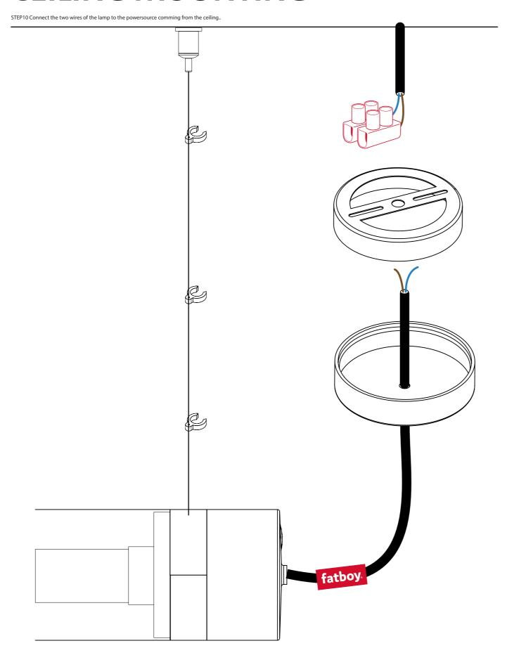
STEP9 Locate the power source and mount the metal cap to cover it. Guide the screw terminal true the big hole.
