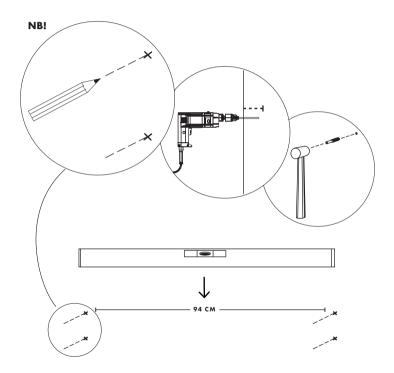
PLACE THE METAL WALL BRACKETS AND SCREW THEM ON TO THE WALL.
