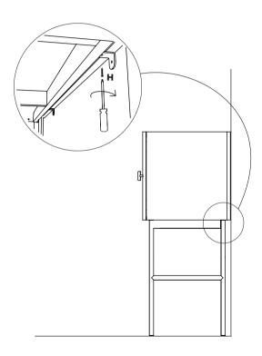
LEVEL, MARK (DISTAINCE 94 CM), DRILL AND USE  $\frac{\text{SUITABLE}}{\text{AND THE SCREWS.}}$  WALL PLUGS
