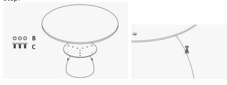
With the help of template screws, place tabletop on metal hardware. Then take out all template screws and install white head screws with washers to combine top and underpart.
