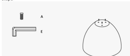
Please install three template screws (nonehead screws) into the underpart.
