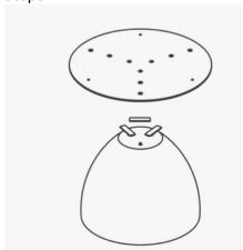
Please put metal hardware on underpart. You can install easily with help of template screws. After place right, please push on the surface. So double adhesives can combine underpart and hardware better.
